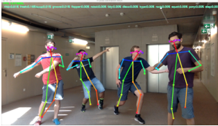
Figure 1: Webcam image overlaid with the output of the pose estimation system along with the estimated probabilities for different dance moves.
