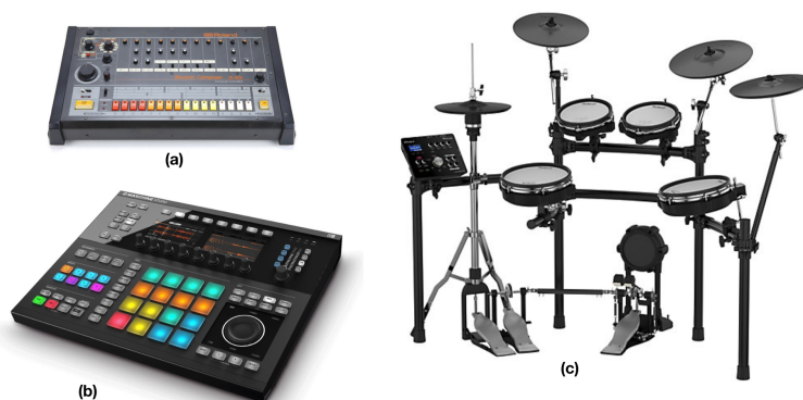
Figure 2.12: Examples of a hardware step sequencer (a) (Roland TR808), hardware MIDI controller featuring pads for finger drumming (b) (Native Instruments Maschine † ), and an e-drum kit (c) (Roland V-Drums ‡ ).
