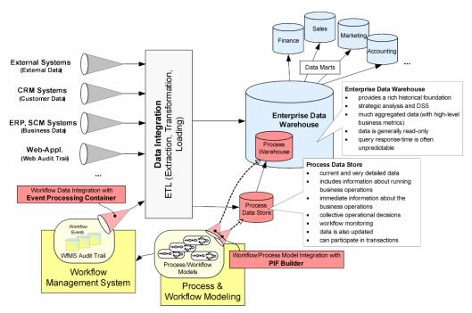
Figure 2. Process information factory - architecture
