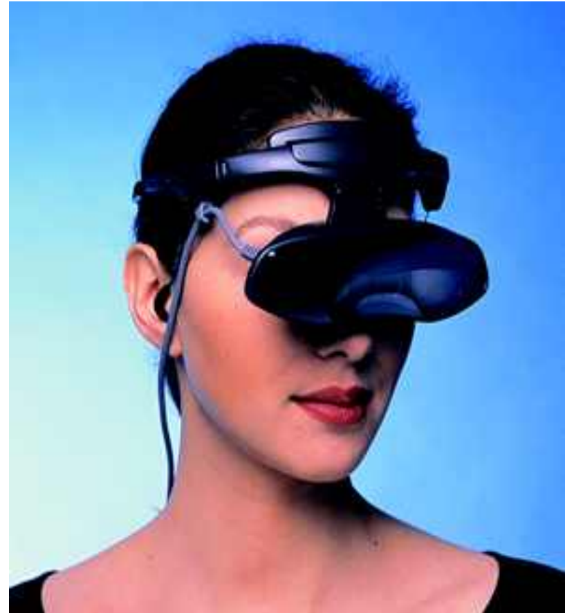
Sony Glasstron (1997-2002): LCD display, Resolution: SVGA (832×624 pixels) FOV: 30 × 22 degrees Weight: 120 grams
