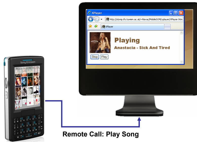
Figure 6.6: XPlayer: The mobile device sends a remote call to play a song which is processed by the XPlayer
