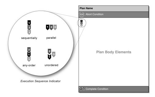
Figure 4: Basic structure and execution sequence symbols.
