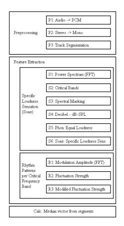
Figure 1: Audio feature extraction block diagram.
